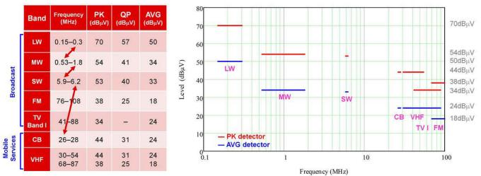
Figure 1. CISPR 25 Class 5 Conducted Emission Limits with Peak (PK) and Average (AVG) Detectors
