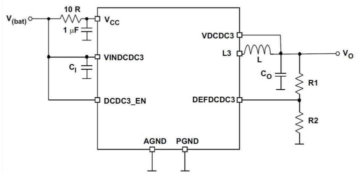
Figure 1. External Enable and Resistor Divider for DCDC3 on the TPS65023
