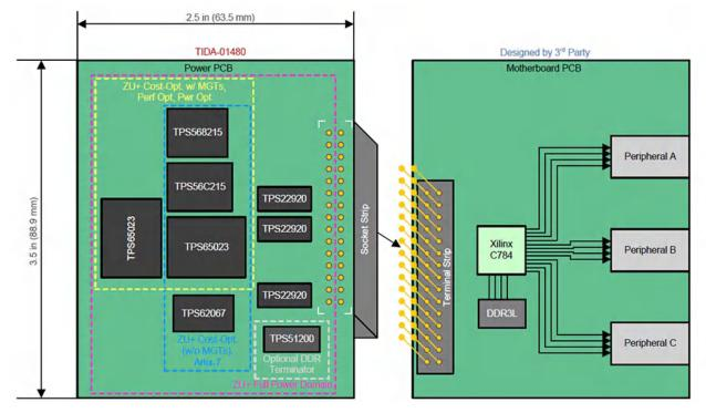
Figure 5. Xilinx Zynq UltraScale+ ZU2CG/ZU5EV MPSoCs Form-factor Conceptual Drawing
