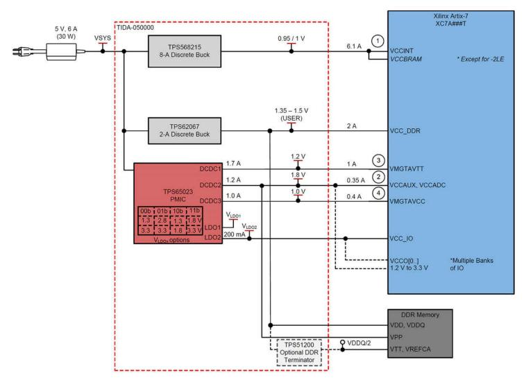
Figure 2. Xilinx Artix-7, Spartan-7 and Zynq-7000 FPGAs Reference Design Block Diagram
