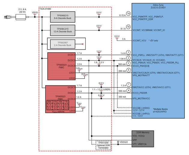
Figure 4. Xilinx Zynq UltraScale+ ZU2CG/ZU5EV MPSoC Block Diagram
