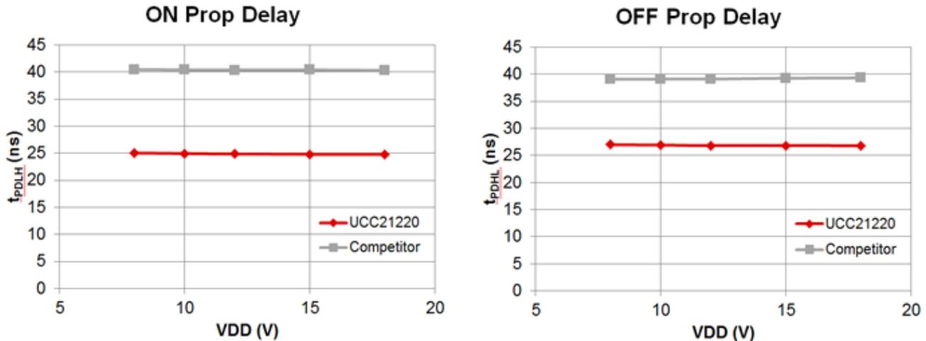
**Figure 2. TI's UCC21220 Propagation Rise/fall Delay with Respect to VDD vs. a Competitor**
