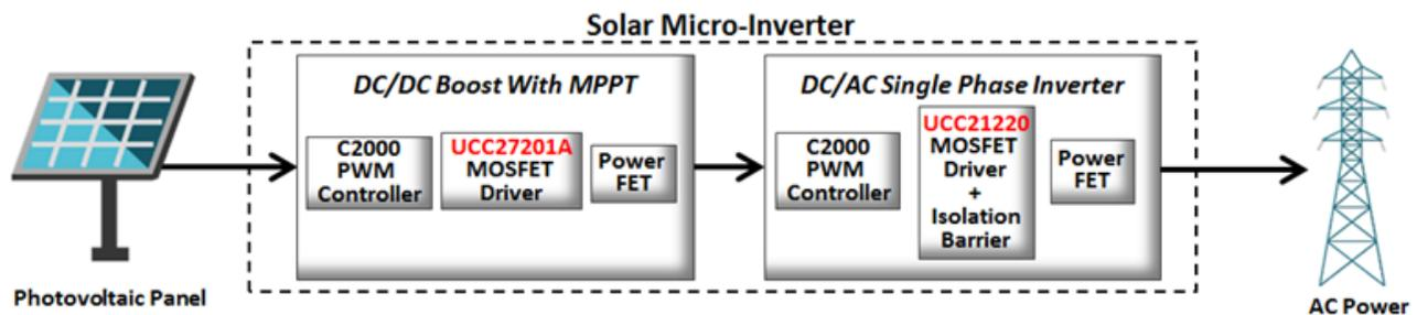
**Figure 1. Typical Solar Microinverter**
