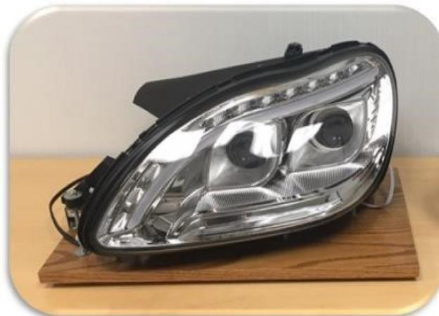
**Figure 3. A Next-generation AFS LED Matrix Headlight Using the TPS92518HV-Q1 and TPS92662-Q1**
