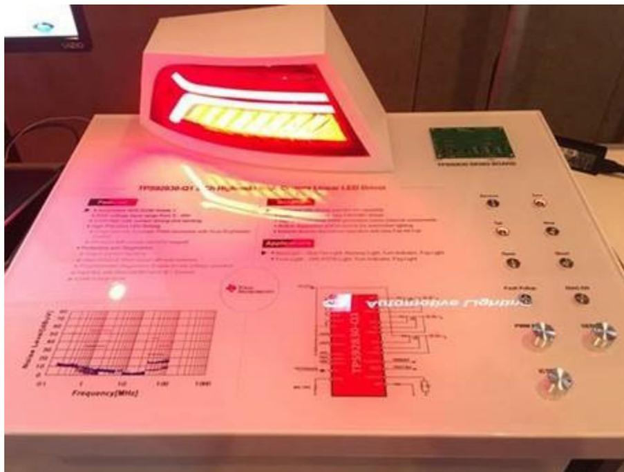
**Figure 1. Automotive RCL Taillight Demo Featuring the TPS92830-Q1 LED Controller**
