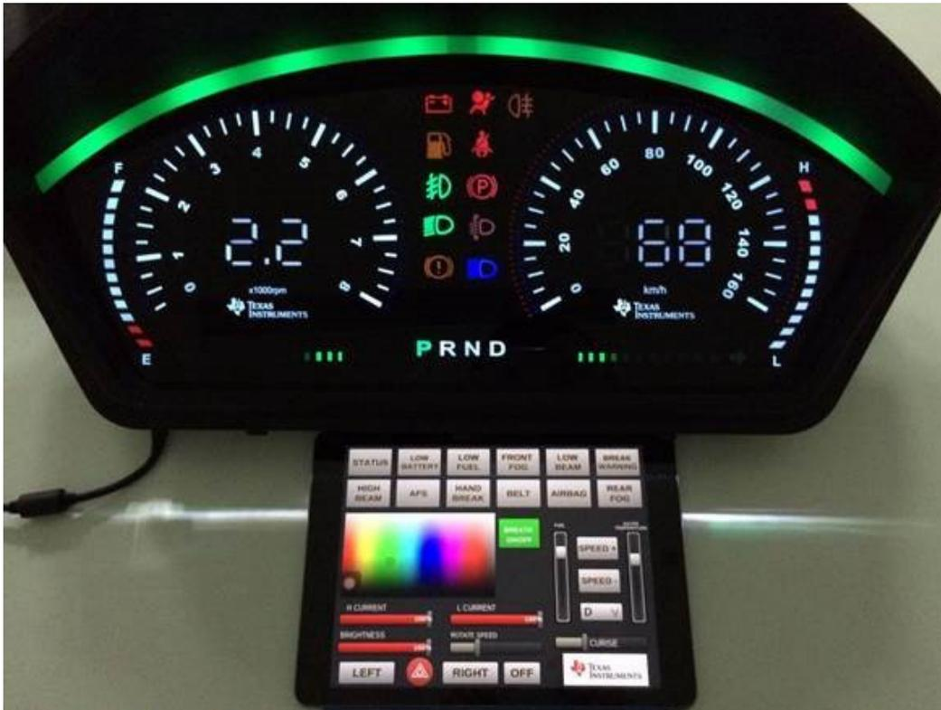
**Figure 2. Sequential/ambient Lighting Using the TLC6C5712-Q1 LED Driver**
