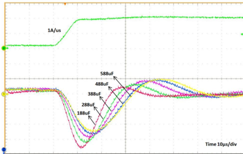
**Figure 4. Transient Response with Different Output Capacitance**
