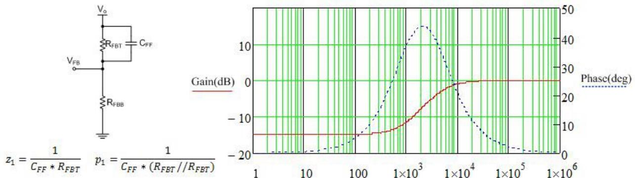
**Figure 1. Feedback Divider with Feedforward Capacitor  $C_{FF}$**
