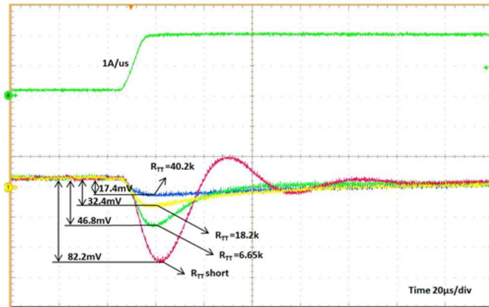
**Figure 5. Transient Response with TurboTrans Technology**
