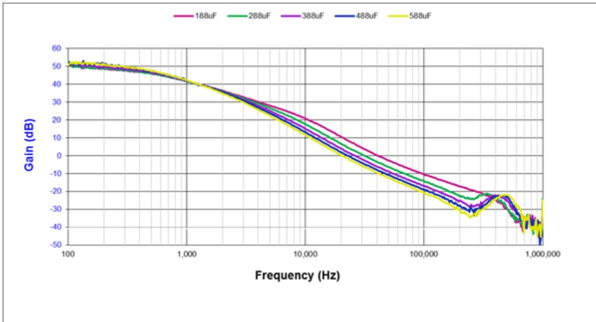
**Figure 3. Gain Curve with Different Output Capacitance**
