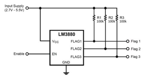
Figure 4. LM3880 Simple Sequencer
