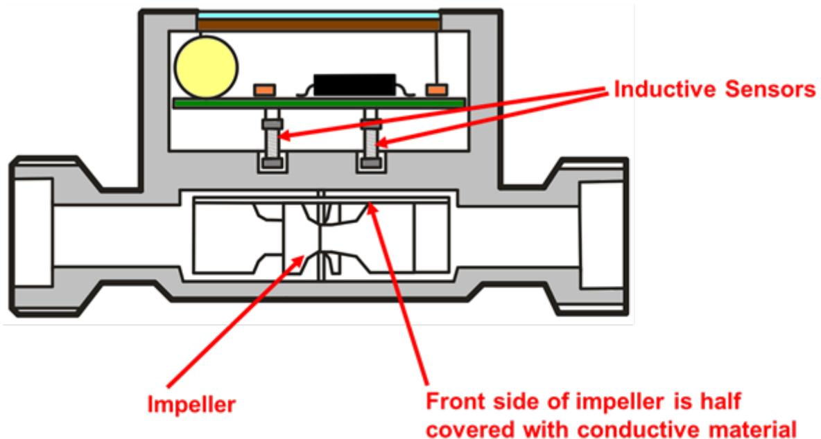
**Figure 2. Rotary-based Flow Meter Using LC Sensors**
