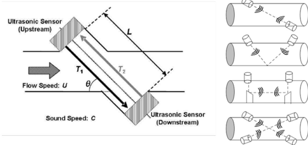
**Figure 3. Examples of Ultrasonic Sensing for Flow Meters and Common Topologies for Positioning within a Pipe**
