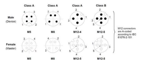
Figure 1. IO-Link SIO Connectors
