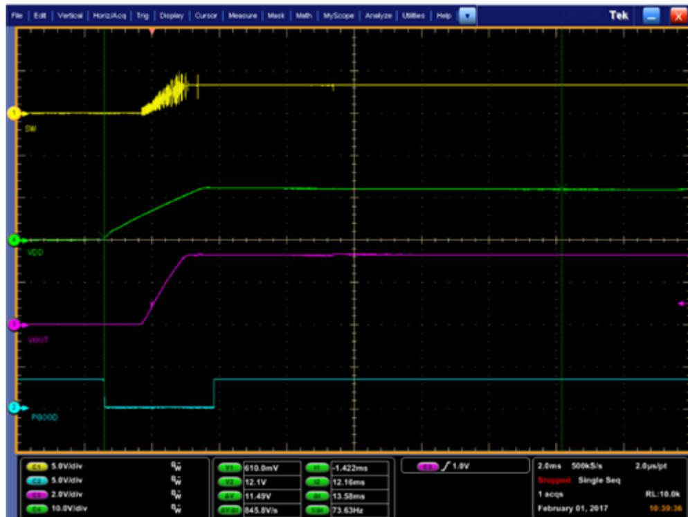
**Figure 5. The TPS53319 Power-good Glitch That Results in an External 3.3V Pull-up on PGOOD Being Present before VDD/VIN**
