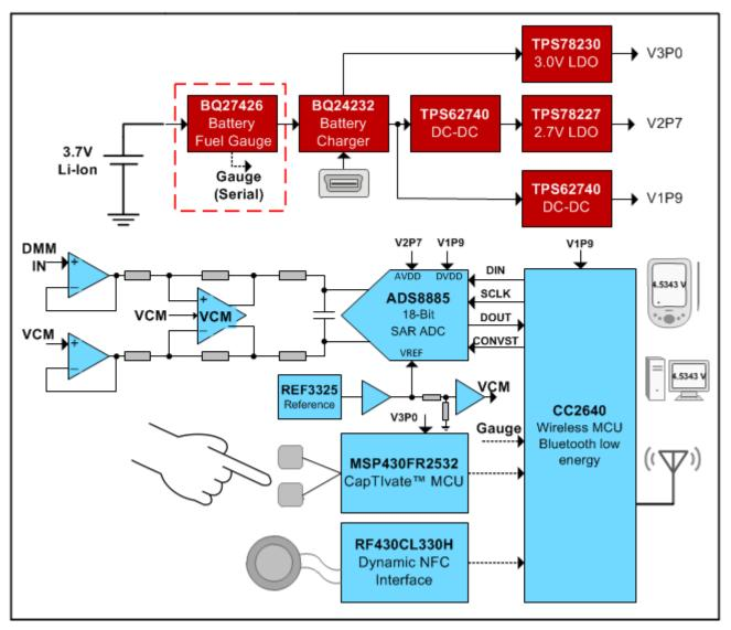
Figure 1. Wireless DMM Block Diagram
