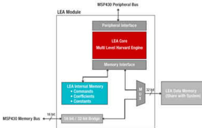
Figure 1. Simplified LEA block diagram
