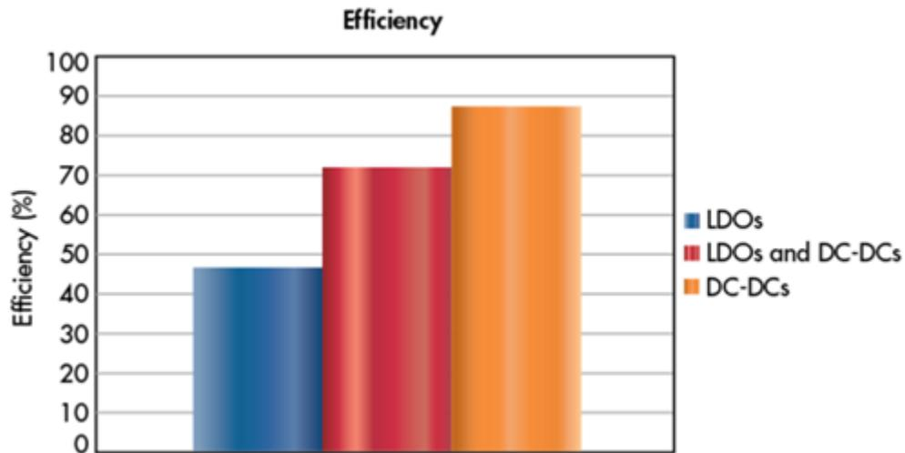
**Figure 3. Efficiency Comparison of Different Power-supply Architectures**
