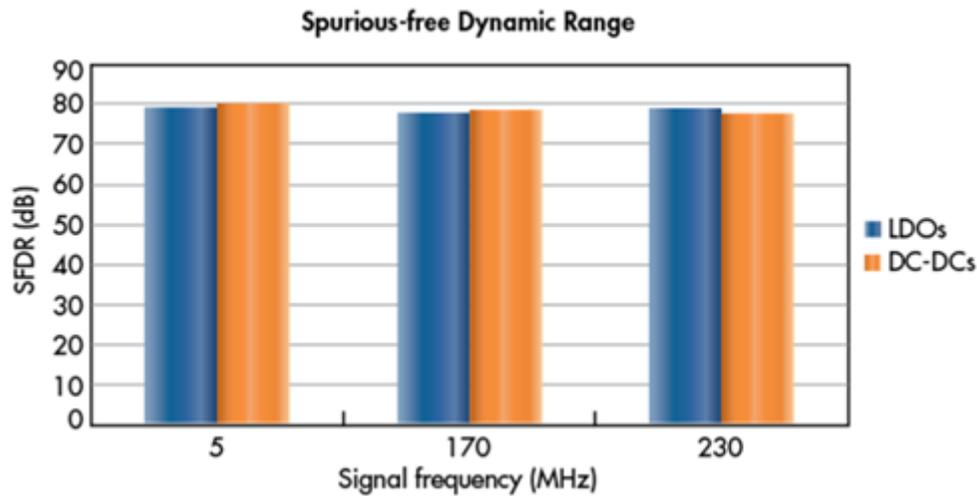
**Figure 2. SFDR of the ADS5407 Powered by LDOs or DC/DCs**
