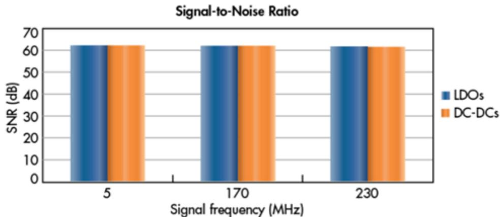
Figure 1. SNR of the ADS5407 Powered by LDOs or DC/DCs
