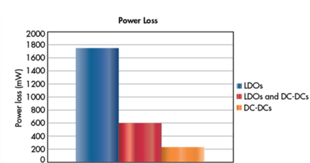
**Figure 4. Power Loss Comparison of Different Power-supply Architectures**
