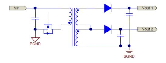
Figure 2. Dual Isolated Outputs with Extra Transformer Winding/rectifier
