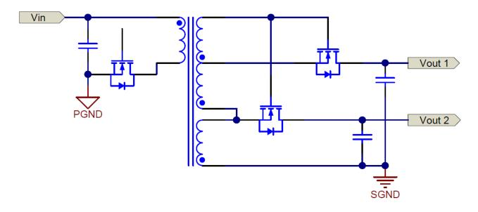
Figure 3. "Self-driven" Method to Control Synchronous FETs
