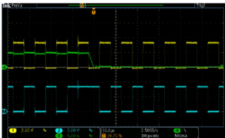
**Figure 1. Self-shutdown of the Power Stage Following a Shoot-through Event (Blue: upper-FET PWM; Yellow: lower-FET PWM; Green: Inductor Current)**
