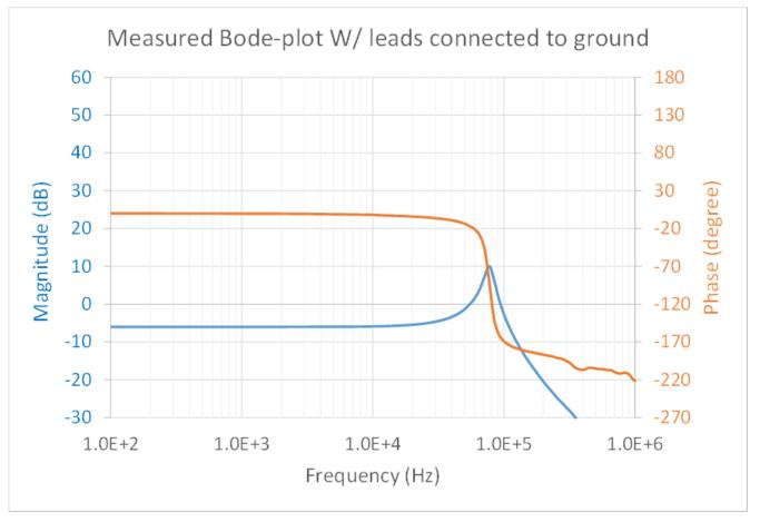
Figure 5. Measured Bode Plot with Reference Leads Connected to Ground
