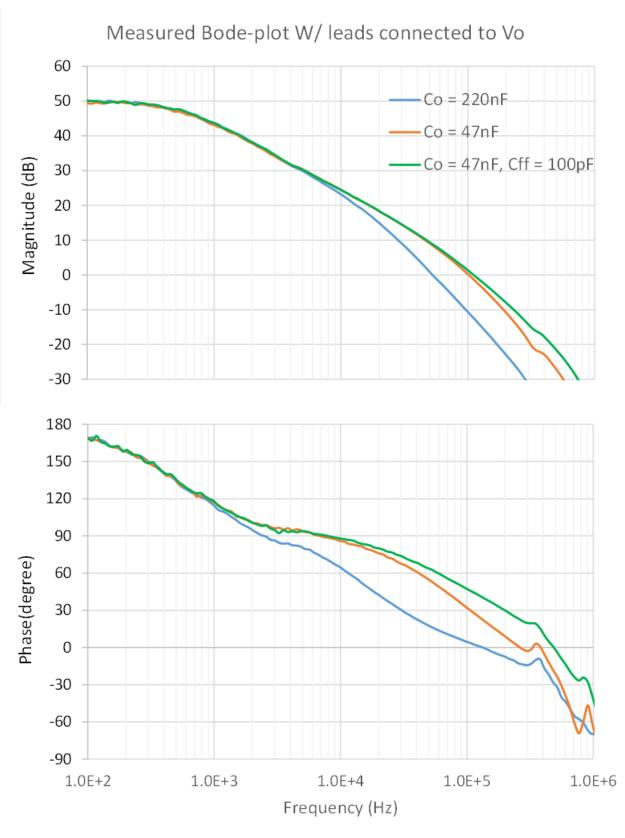
Figure 10. Measured Bode Plot with a Different Co and Cff
