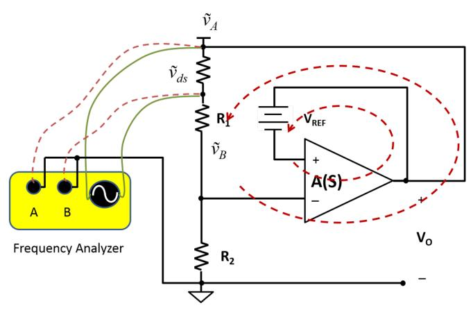
Figure 6. Small-signal Model Referring to Ground
