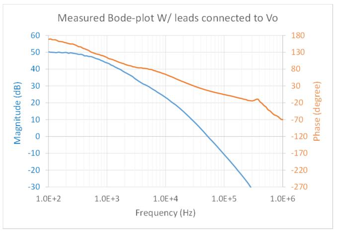
Figure 8. Measured Bode Plot with Reference Leads Connected to vo
