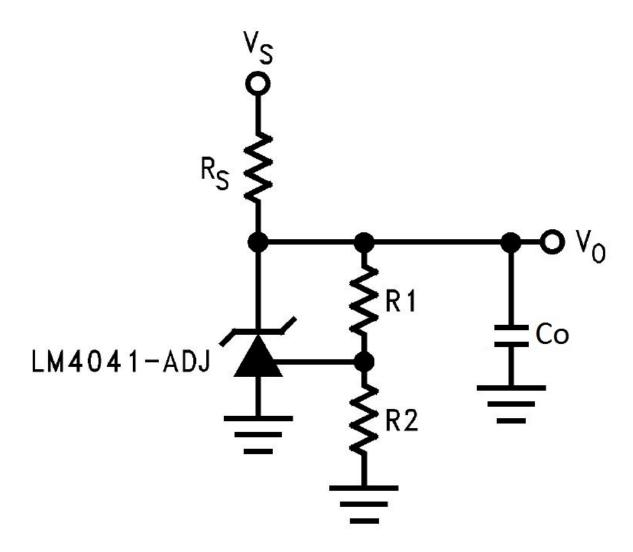
Figure 3. LM4041-N Typical Application Circuit
