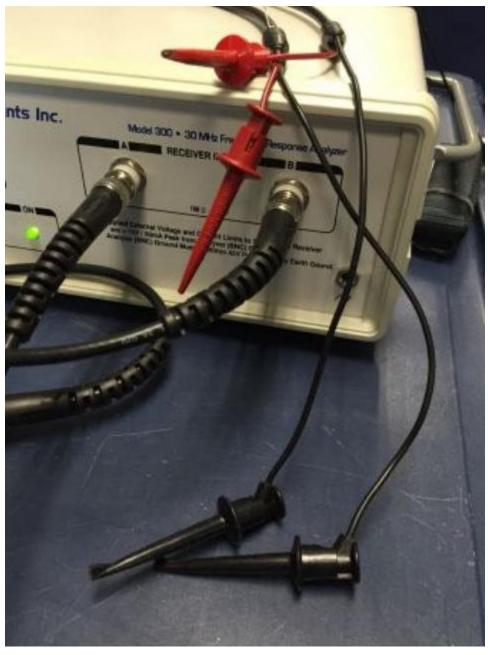
Figure 2. Probes of Receivers a and B with Their Reference Leads
