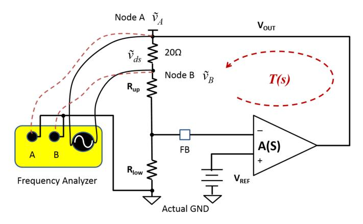
Figure 1. Typical T Measurement Setup
