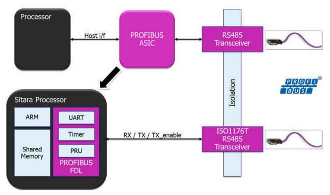
Figure 2. Integrating the PROFIBUS function of an external ASIC into the Sitara processor
