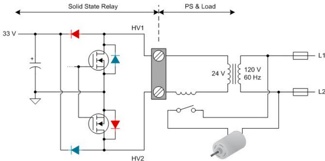
**Figure 2. Power Supply of an SSR in an HVAC System**
