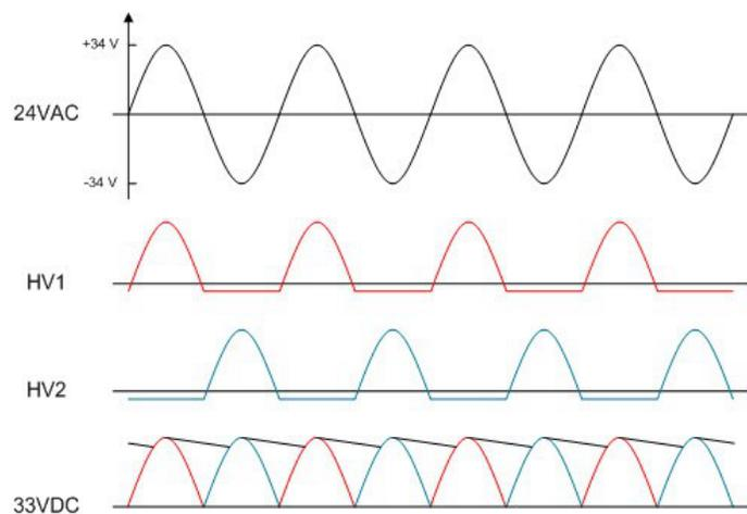
**Figure 3. Full-wave Rectification Waveforms**
