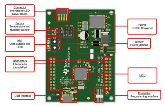
Figure 2. Power and Control Board
