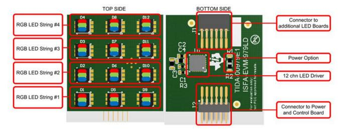
Figure 3. LED Driver and Red/green/blue LEDs
