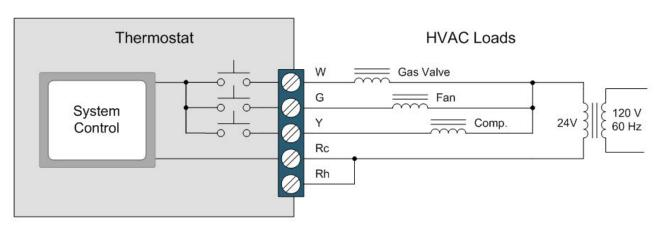
Figure 2: Functional diagram of a basic thermostat
