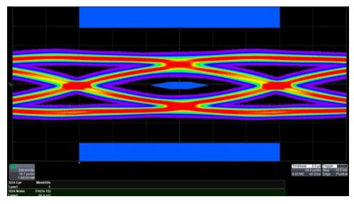
Figure 2. USB 3.1 Gen 2 Eye Diagram (with the TPD4E02B04)
