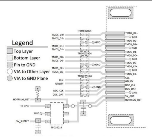
Figure 4. HDMI 2.0 Type-A Transmitter Port Layout
