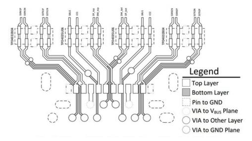
Figure 5. USB Type-C Mid-mount Hybrid Connector with One-sided ESD Layout
