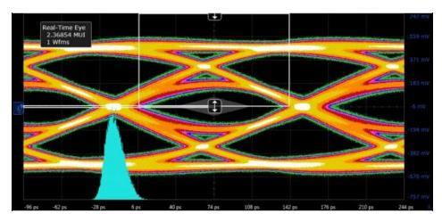
Figure 3. HDMI 2.0 6Gbps TP2 Eye Diagram (with the TPD4E02B04)
