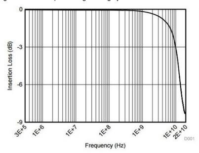
Figure 1. TPD4E02B04 Differential Insertion Loss
