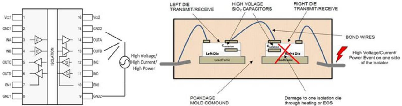
**Figure 2. Failure Mode 2 Is High Voltage and High Current Close to an Isolation Barrier**
