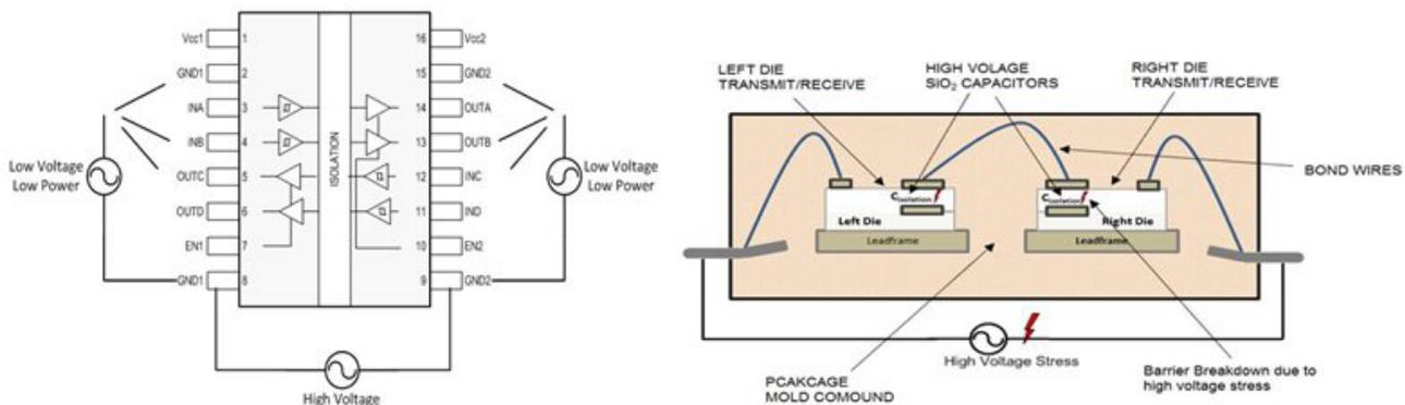
**Figure 1. Failure Mode 1 is a High Voltage across the Isolation Barrier**
