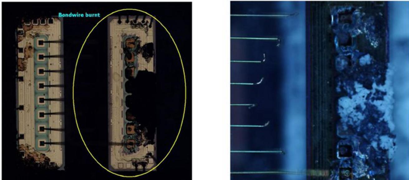
**Figure 3. TI-reinforced Isolators Survive Failure Mode 2**
