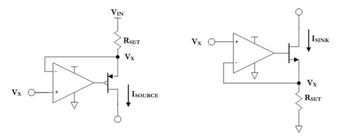
Figure 1. Feedback-generated Current Source and Sink Circuits
