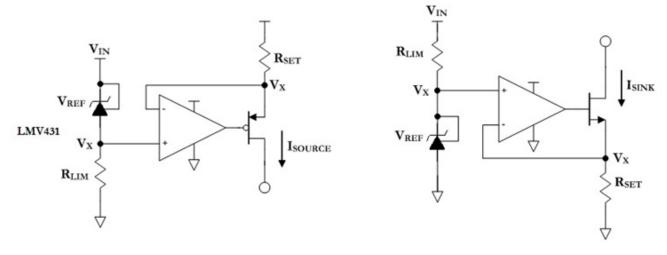
Figure 2. Feedback-generated Current Source and Sink Circuits
