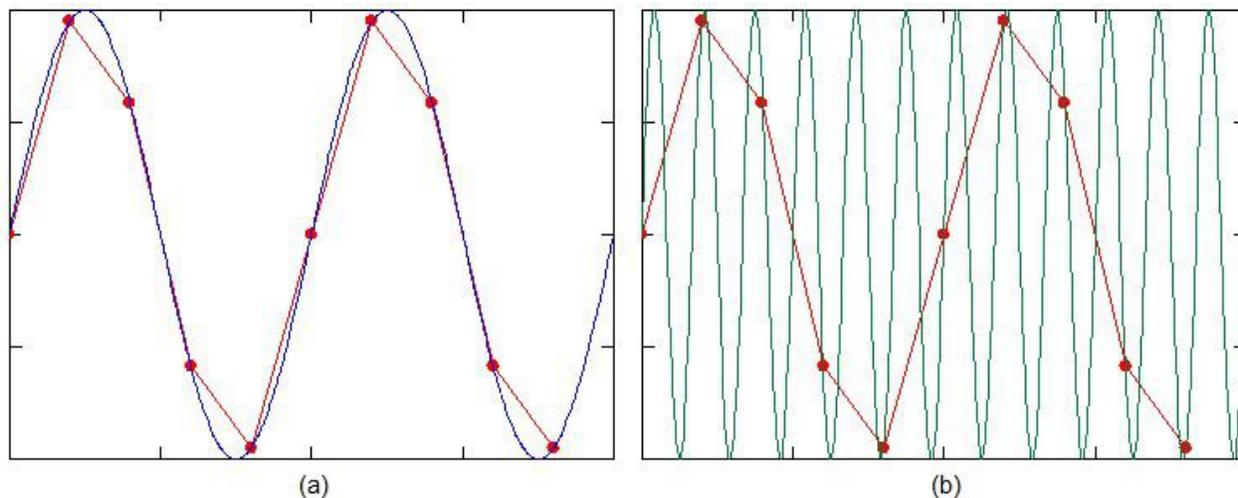
**Figure 1. (a) Sinusoid Signal with Discrete Sampling and (b) Visualization of Higher-frequency Aliasing**
