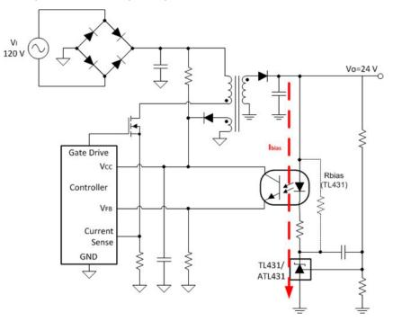
Figure 1. General Schematic of a Flyback Power Supply
