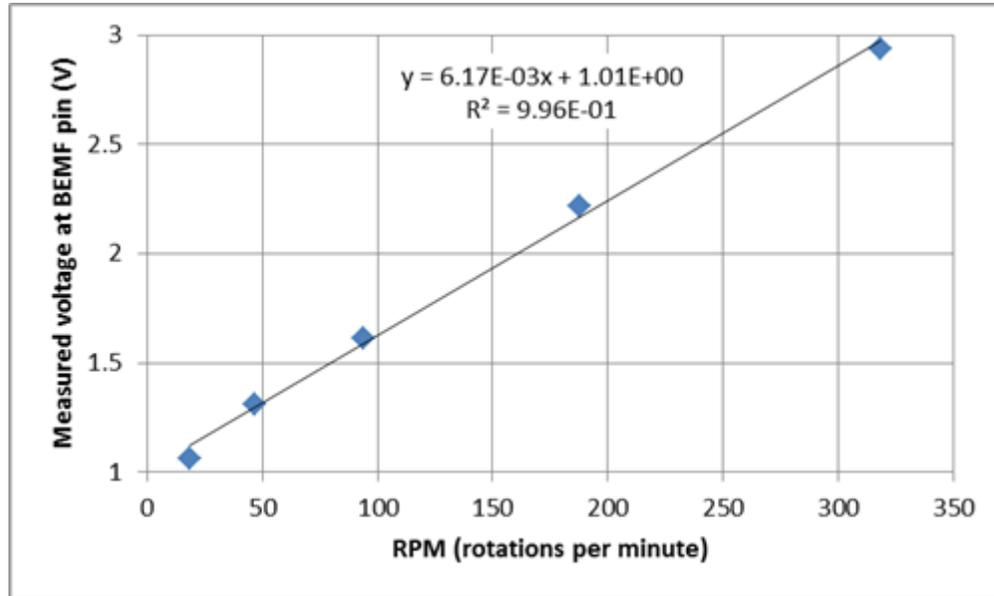
**Figure 5. A Few Points of Back EMF Data: It's Pretty Linear with Motor Speed**
