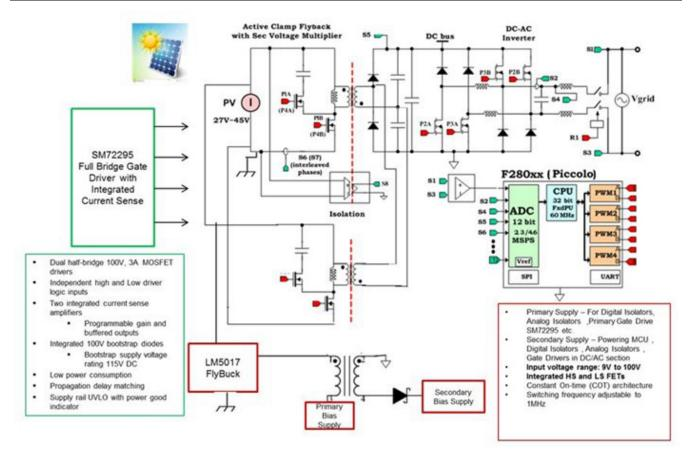
Figure 4. DC/DC Section of Grid Tie Microinverter
