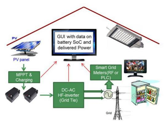
Figure 1. Smart Connected Home with Renewable Power Storage
