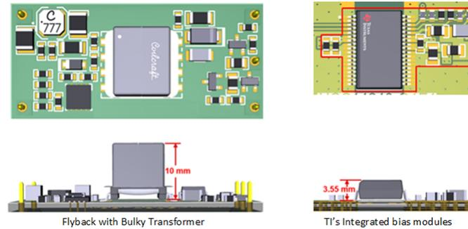
**Figure 1-5. A TI isolated bias module vs. flyback size and component comparison**
