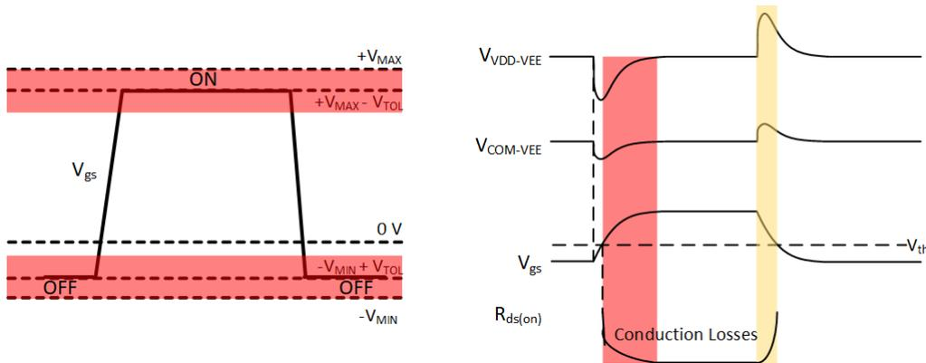
**Figure 1-4. SiC gate-source voltage limits and conduction losses during a switching cycle**
