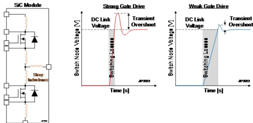
**Figure 1-2. SiC slew-rate control by varying gate-driver IC drive strength**
