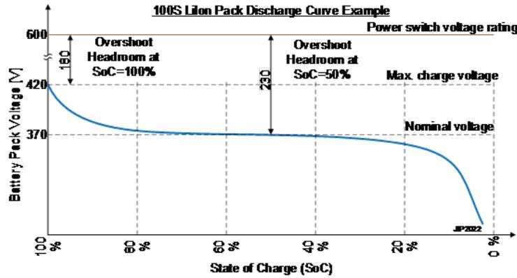
**Figure 1-3. Efficiency zone during battery peak voltage vs. state of charge**
