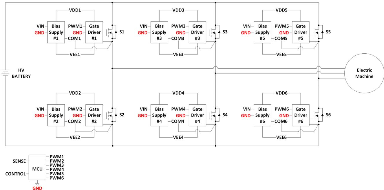
Figure 1-1. EV traction inverter block diagram
