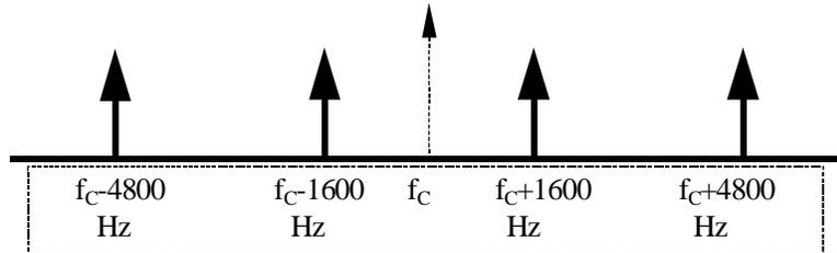
Figure 5 shows a typical 4 Level FSK output function of a discriminator type demodulator. The discriminator demodulation technique outputs an audio frequency signal. With this technique the output amplitude is proportional to the input frequency deviation.
