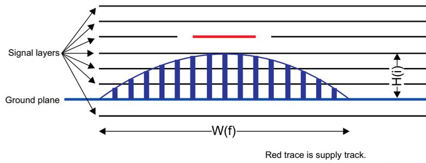
**Figure 5. Frequency/Current Impact On Ground Plane**
