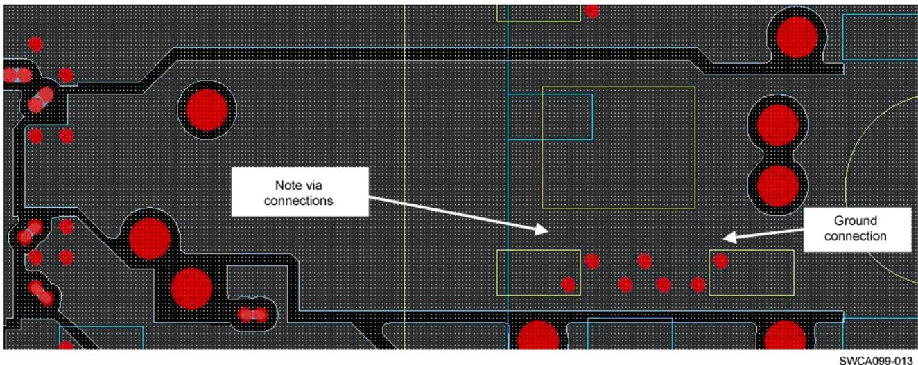
Figure 12. DC/DC Routing on GND1 Layer
