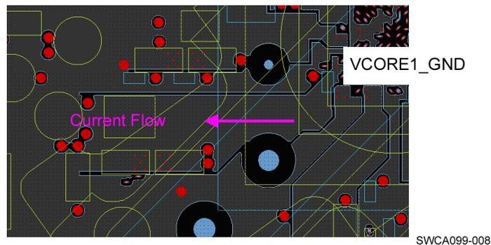
Figure 7. Zoom on SMPS VCORE1 Ground Plane
