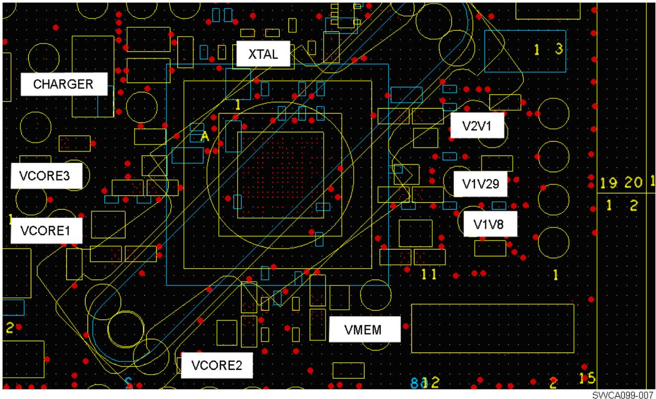
Figure 6. Example of Component Placement on SELAB Daughterboard
