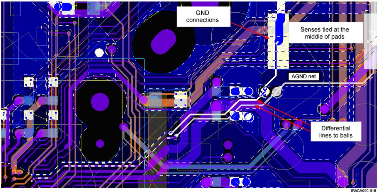
Figure 17. Fuel Gauge Sense Resistor Routing
