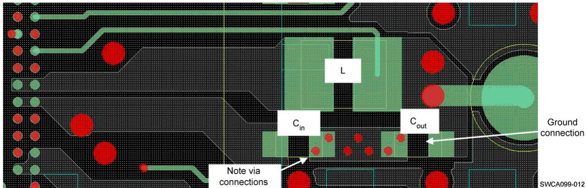
Figure 11. DC/DC Routing on Top Layer
