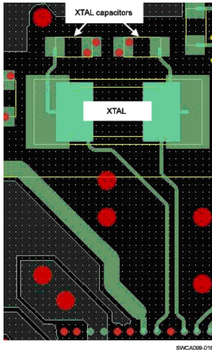
**Figure 15. Crystal Components Placement**
