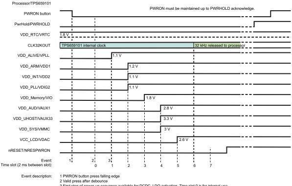
3 First step of power-up sequence available for DCDC, LDO activation. Time slot 0 is for internal use. Note: PWRON press must be maintained until PWRHOLD acknowledge, or, for shorter PWRON press, PWRHOLD must go high within 984 ms of valid PWRON press (event 2).
