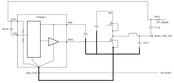
Figure 14. DC/DC Controller Remote Sensing
