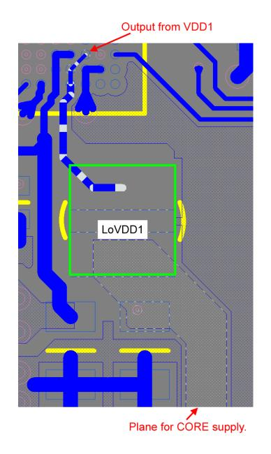
Figure 11. Badly Routed DC/DC Switching Load
