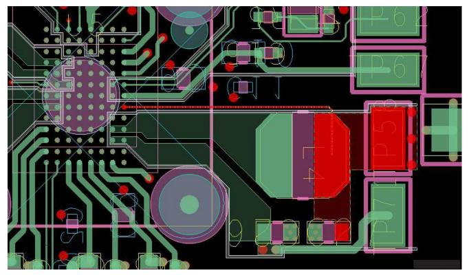
Figure 10. Badly Routed Feedback on DC/DC Converter
