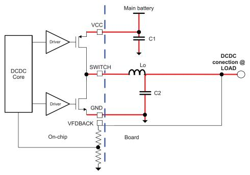
Figure 7. DC/DC Converter
