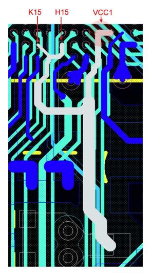
Figure 9. Badly Routed Supply Connections
