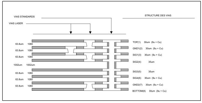
Figure 3. Evaluation Board PCB Layer Information
