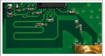
Figure 2 Layout of transmission line implementation
