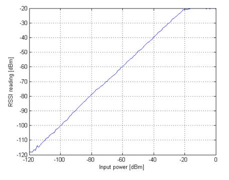
Figure 3. Typical RSSI vs Input Level, HGM, 50 kbps
