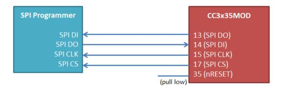
Figure 5. Programming Through SPI
