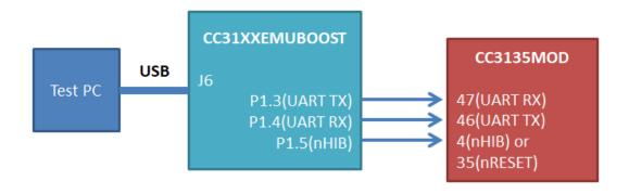
Figure 4. Programming Through USB
