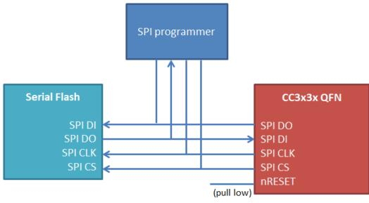
Figure 4-1. Programming Through SPI
