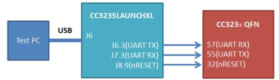
Figure 5-1. Connecting Through USB
