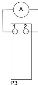
**Figure 4: Connector P3 with ampere meter attached**
