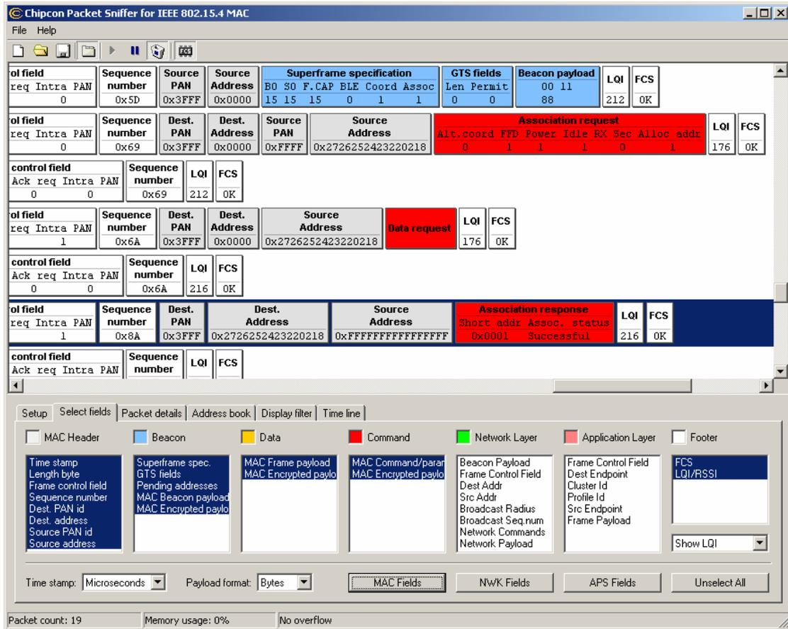
**Figure 7: Packet Sniffer Capture Window**
