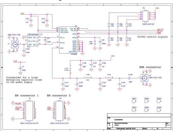
Figure 3. CC2592EM Schematic Diagram
