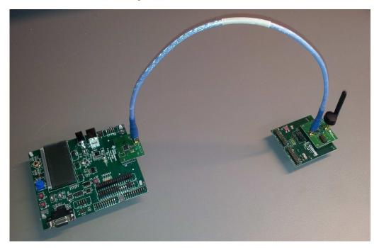
Figure 2. Possible SetUp of CC2592 + Radio (no control signals)
