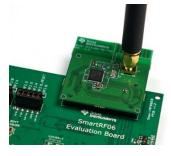
Insert a CC1310EM board into a SmartRF06EB and connect the antenna to the SMA connector on the EM. Note that the PCB antenna on the board can be used instead of the whip antenna. Refer to the CC1310 schematics to see how to enable it.
