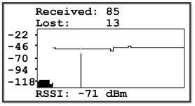
In RX mode, the LCD displays the number of received packets, lost packets, and RSSI as shown above.
