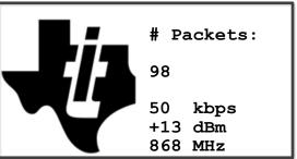
Running TX mode will transmit packets at a given rate. The LCD will show the number of packets transmitted together with info about the test case, output power (rounded) and frequency band.
