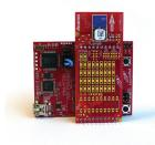
The RF BoosterPack includes an ETSI-compliant and FCC certified module integrating TI's CC110L sub-1 GHz RF value line transceiver, passive components and compact PCB antenna. For more information, visit www.ti.com/rfboosterpack
