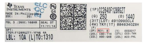
Figure 3. Sample Product Shipping Label for the CC2640 Device
