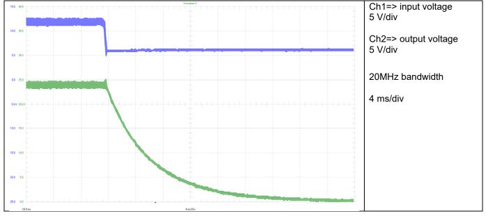
Figure 25 Shutdown with 12 V Input Voltage
