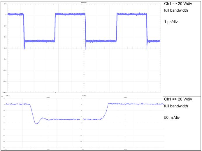
Figure 14 Diode D1 at 24 V Input Voltage
