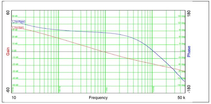
Figure 18 Bode Plot for 7 V Input Voltage
