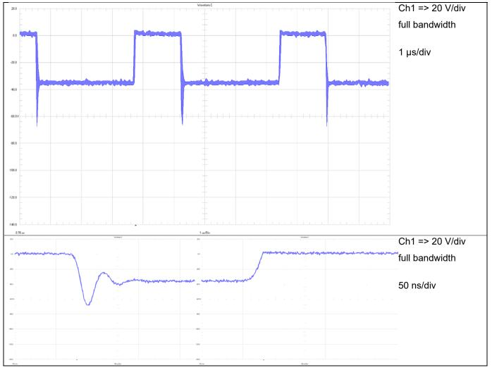
Figure 13 Diode D1 at 12 V Input Voltage
