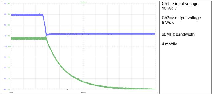
Figure 26 Shutdown with 24 V Input Voltage
