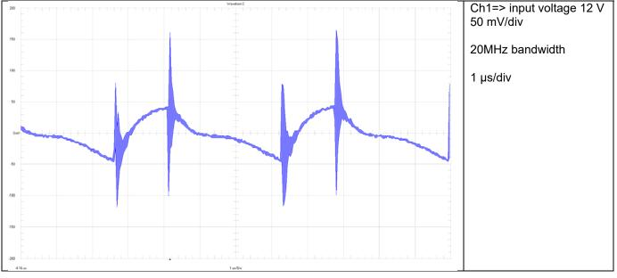
Figure 16 Input Ripple Voltage (12V Input Voltage)
