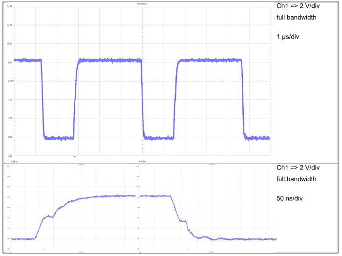
Figure 11 Q1 Gate at 12 V Input Voltage
