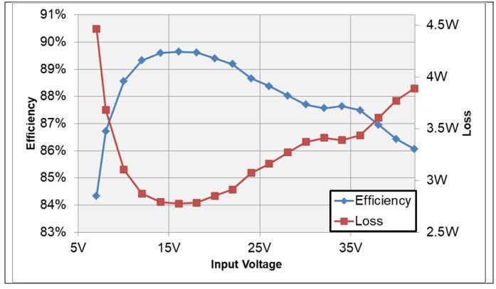
With the same setup efficiency and loss were calculated.
