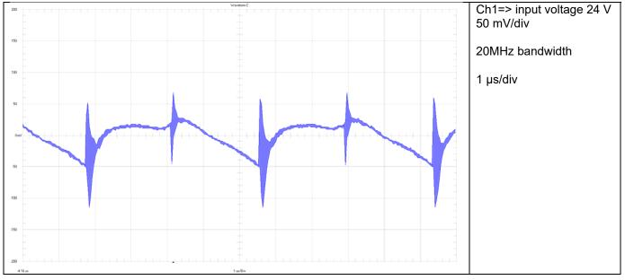
Figure 17 Input Ripple Voltage (24 V Input Voltage)
