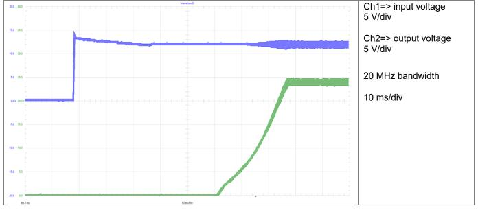
Figure 23 Start-Up with 12 V Input Voltage
