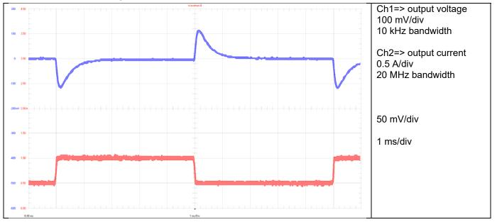
Figure 21 Load Transient with 12V Input Voltage
