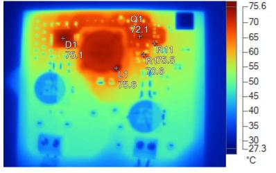
Figure 6 IR Photo for 12 V Input Voltage
