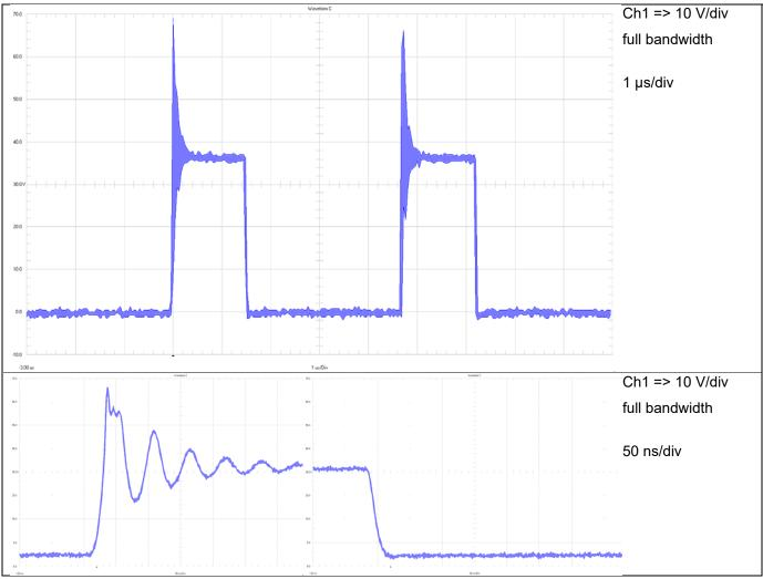
Figure 9 Switchnode Q1 at 12 V Input Voltage
