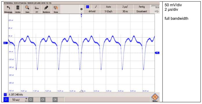
Figure 6 Output Voltage Ripple
