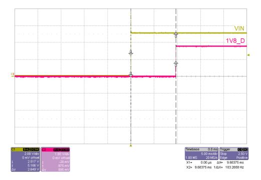
The photo below shows the output voltage startup waveform after the application of 5V in on the VIN rail with the 12V output rail loaded to 0A. (12V: 5V/DIV, 10mS/DIV), (VIN: 2V/DIV)
