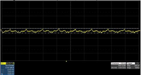
The output ripple voltage is shown in the figure below. The image was taken with the 12V output loaded to 0.06A and the input voltage VBAT set to 4.1V. (10mV/DIV, 1uS/DIV)
