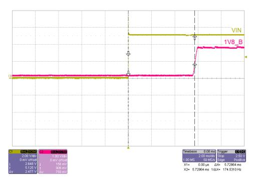
The photo below shows the output voltage startup waveform after the application of 5V in on the VIN rail with the 1V8\_C output rail loaded to 0A. (1V8\_C: 1V/DIV, 5mS/DIV), (VIN: 2V/DIV)
