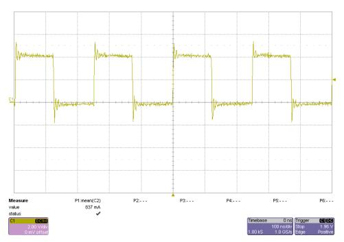
The photo below shows the switch node voltage. The input voltage VBAT is 4.1V and the 1V8\_C output is loaded to 0.3A. (2V/DIV, 500nS/DIV)
