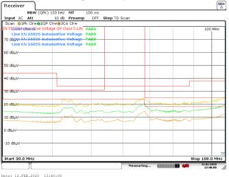
13VIN, 5V/2.5A, 1.1V/2.2A, 3.3V/1.65A, 1.8V/0.18A, 30MHz to 108MHz (measured at low side LISN)
