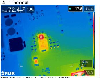
12Vin, 5V/2.5A, 1.1V/2.2A, 3.3V/1.65A, 1.8V/0.18A, Tmax(U1)=72.4C, Room Temp, Natural Convection
