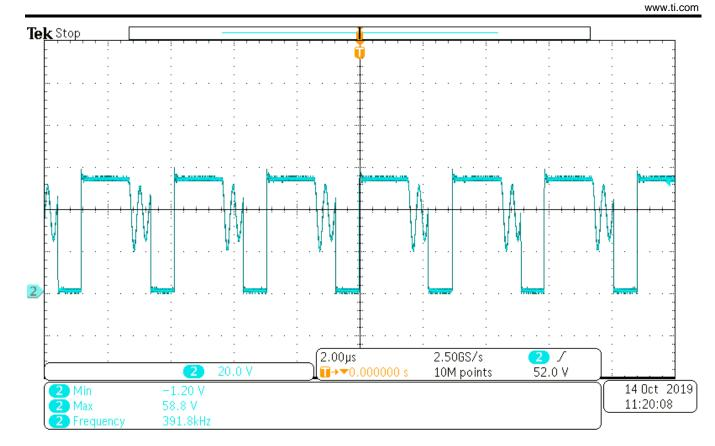
• CH2: Switching node at 36.0V in and 0.1A load current on both outputs [scale: 20.0V/div, 2.0us/div]
