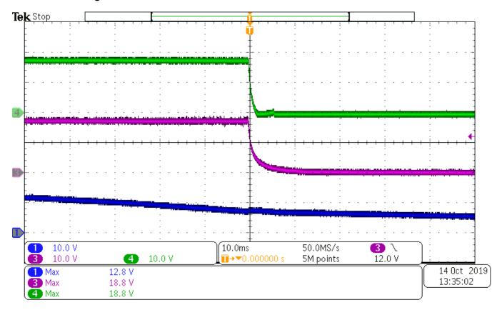
• CH1: Input voltage at 12.0V in and 0.1A load current on both outputs [scale: 10.0V/div, 10ms/div]
