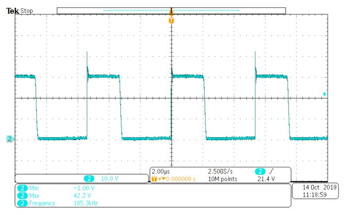
• CH2: Switching node at 12.0V in and 0.1A load current on both outputs [scale: 10.0V/div, 2.0us/div]
