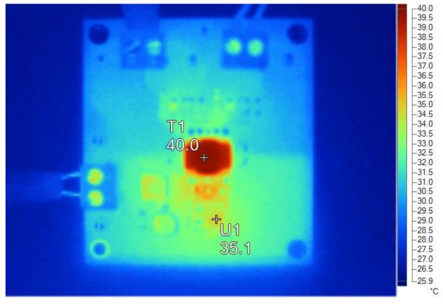
Thermal image of the PCB's top side at 12.0V in and 0.1A load current on both outputs.
