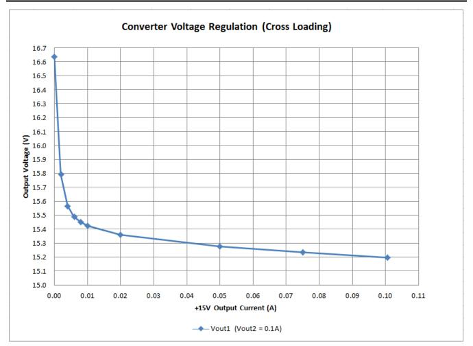
Figure 3-4. Output Voltage Regulation With Cross Loading
