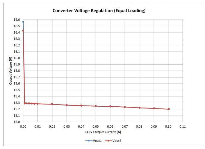
Figure 3-3. Output Voltage Regulation With Equal Loading
