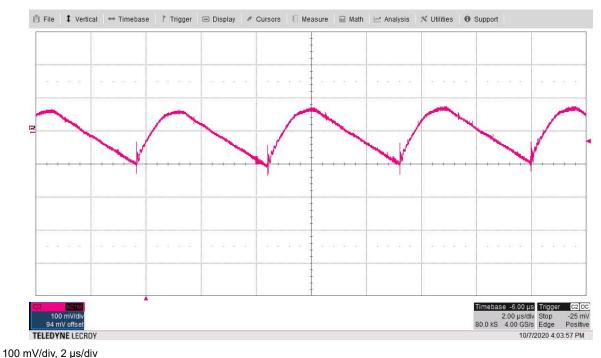
Figure 4-12. Ripple Voltage, 15-V Output
