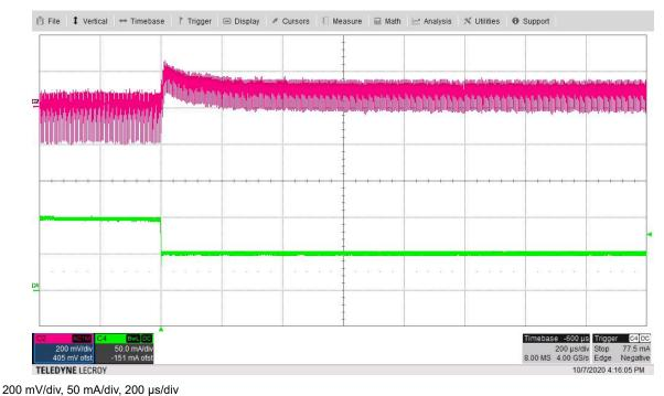
Figure 4-15. Load Transients, 15-V Output Voltage
