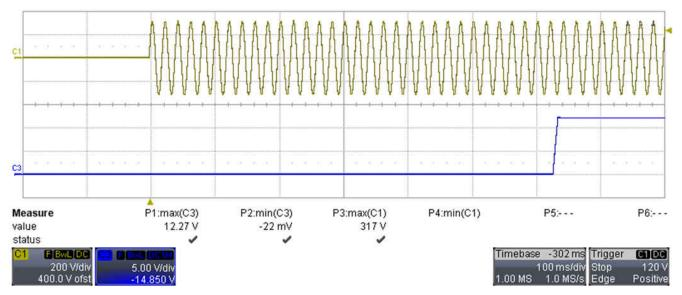
Figure 3-6. Start-Up With 0-A Load (100 ms/div)
