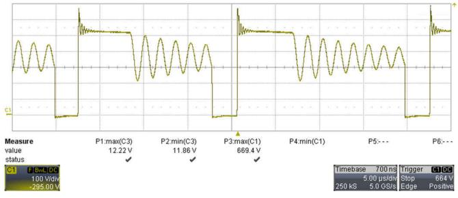
Figure 3-1. Waveform Q1-V<sub>DS</sub> (100 V/div, 5 µs/div, 200 MHz BWL)
