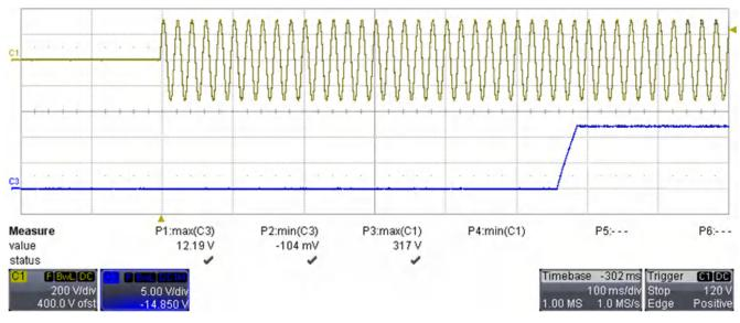
Figure 3-8. Start-Up With 1.7-A Load (100 ms/div)
