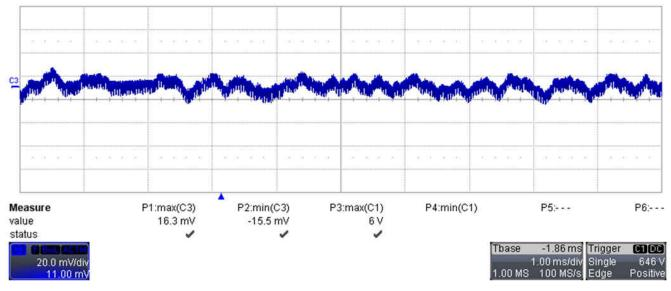
Figure 3-4. Output Voltage (20 mV/div, 1 ms/div, AC coupling)
