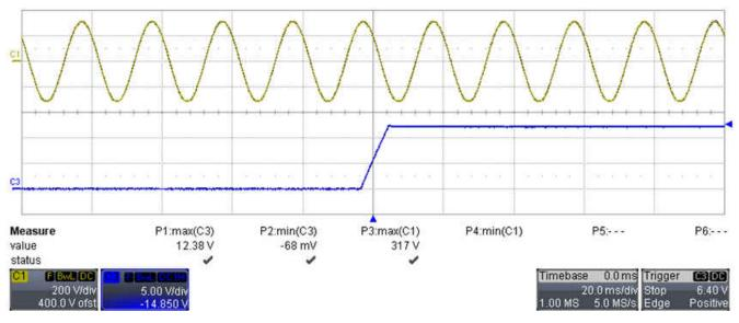
Figure 3-7. Start-Up With 0-A Load (20 ms/div)
