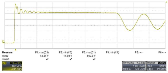
Figure 3-2. Waveform Q1-V<sub>DS</sub> (100 V/div, 1 µs/div, 200 MHz BWL)
