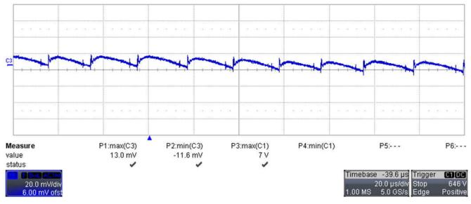
Figure 3-3. Output Voltage (20 mV/div, 20 µs/div, AC coupling)
