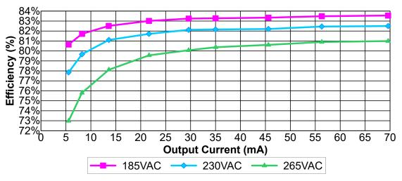
Figure 2-1. Light Load Efficiency
