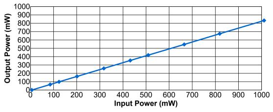
Figure 2-2. Output Power vs Input Power
