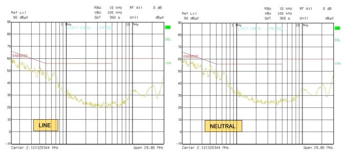
Figure 2-7. EMI: V<sub>IN</sub> = 230 V<sub>AC</sub>, R<sub>LOAD</sub> = 7.06 Ω, Negative Output Terminal Connected to LISN Ground
