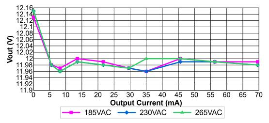
Figure 2-5. Output Voltage vs Output Current (Light Load)
