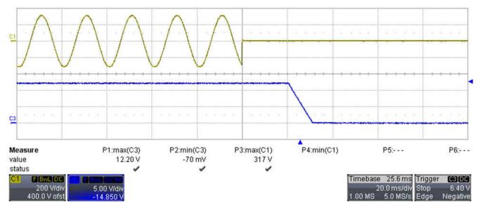
Figure 3-10. Shutdown Sequence With 1.7-A Load Current
