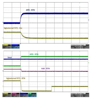
Figure 3-15. PSE Voltage = 48V, Adapter Voltage = 40V, Load = 3A
