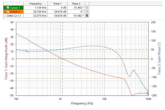
Figure 2-6. 3A Load Bandwidth = 1.134kHz, Phase Margin = 51.462Degrees, Gain Margin = 26.676dB
