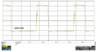
Figure 3-5. Voltage Drain-to-Source, Q10, 37V Input, 3A Load, Measured 136.7V V<sub>peak</sub>
