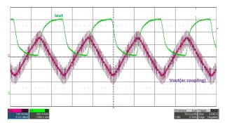
Figure 3-9. Output Load Step Response, 1.5A to 3.0A Load Step
