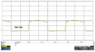
Figure 3-4. Voltage Drain-to-Source, Q8, 57V Input, 3A Load, Measured 52.5V  $V_{\text{peak}}$
