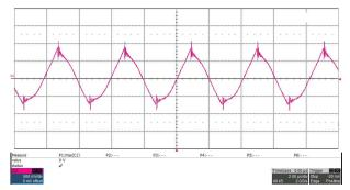
Figure 3-7. DC/DC Converter Input Voltage Ripple
