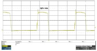
Figure 3-3. Voltage Drain-to-Source, Q8, 37V Input, 3A Load, Measured 105.8V V<sub>peak</sub>
