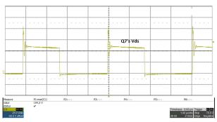
Figure 3-2. Voltage Drain-to-Source, Q7, 57V Input, 3A Load, Measured 104.2V V<sub>peak</sub>
