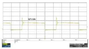
Figure 3-1. Voltage Drain-to-Source, Q7, 37V Input, 3A Load, Measured 69.2V V<sub>peak</sub>
