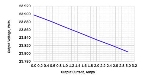
Figure 2-2. Load Voltage Regulation Curve
