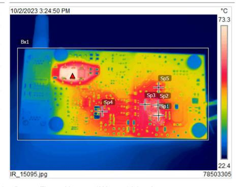
Figure 2-4. Bottom Thermal Image, 48V Input, 3A Load
