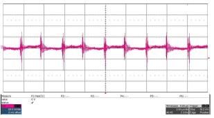
Figure 3-8. Output Voltage Ripple
