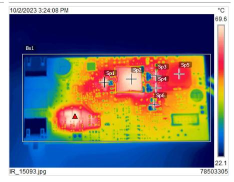
Figure 2-3. Top Thermal Image, 48V Input, 3A Load
