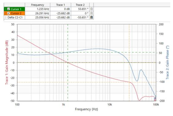
Figure 2-5. 0A Load Bandwidth = 1.235kHz, Phase Margin = 53.651Degrees, Gain Margin = 25.682dB
