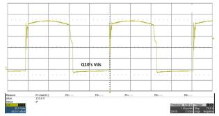
Figure 3-6. Voltage Drain-to-Source, Q10, 57V Input, 3A Load, Measured 110.0V V<sub>peak</sub>
