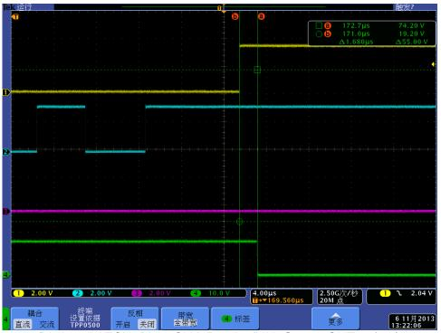
(Yellow: LATCH; Blue: CLK; Purple: DIN; Green: OUT4 of #1) Fig 9, Delay between the rising edge of LATCH and outputs updated
