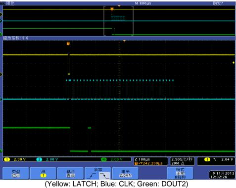
Fig 3, Example of read back OCP fault (Set outputs ON first).
