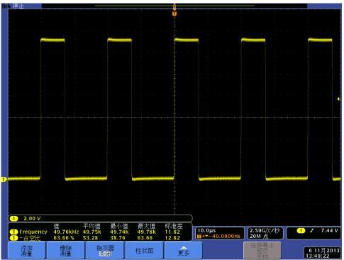
Fig 15, Output voltage - set to 62.5% PWM duty (50kHz)
