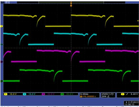
(Yellow: OUT1 #1; Blue: OUT2 #1; Purple: OUT3 #1; Green: OUT4 of #1) Fig 21, Half step commutation output pattern with stepper connected
