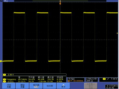
Fig 14, Output voltage – set to 50% PWM duty (50kHz)
