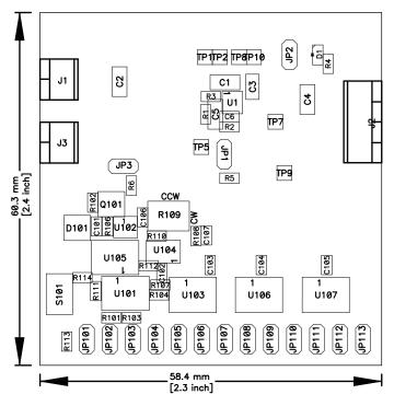
Figure 6. Assembly Layer
