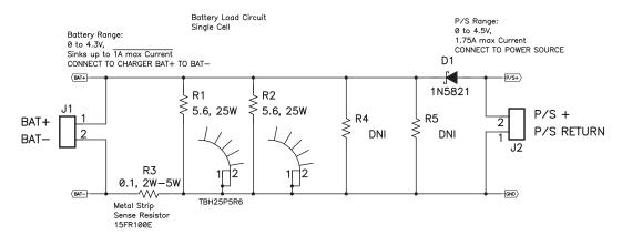
Figure 3. Battery cell Replacement – Allows quick battery adjustment
