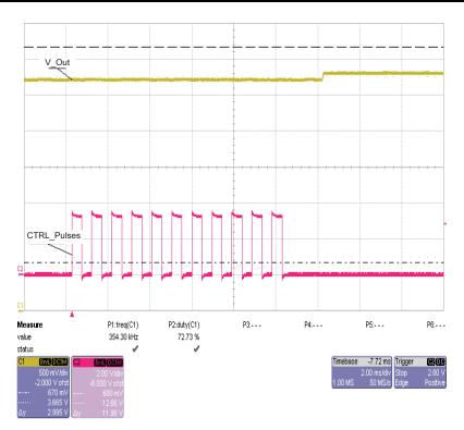
Figure 2. Pulse Programming – CH2: 11 pulses; CH1: V<sub>OUT</sub> IR change due to increased charge current.
